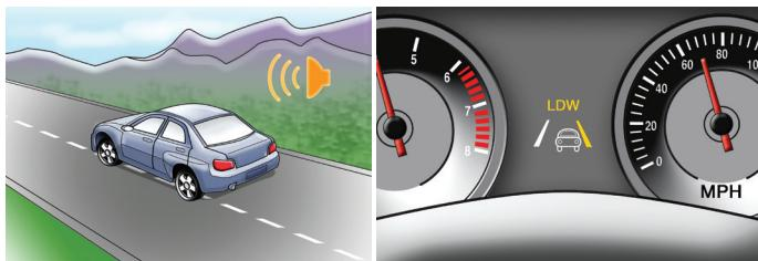
Some vehicles are equipped with lane keeping assist, which is a more advanced version of lane departure warning. If the system detects a potential lane departure and you do not respond in time, lane keeping assist will gently steer you back into the lane.
